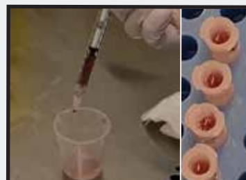
Staining with 0.2 ml nanoreagent on the filter, followed by 10 min incubation to allow nanoparticles binding
